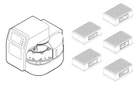
Place tip combs on Lysis plate or in dedicated tip plate, according to machine's specifications.
