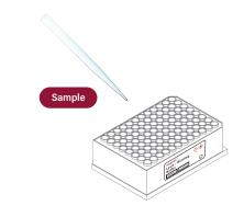
Peel remaining three plates and load all plates onto their respective positions on the extraction machine.
